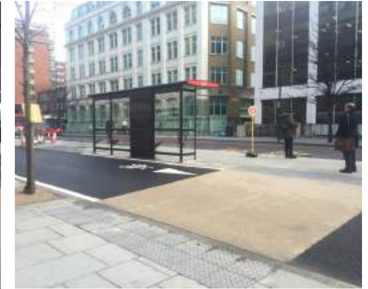
Asphalt Cycle Track / Clearly identifiable as a movement corridor with buff pedestrian crossing
