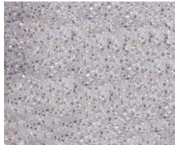
Precast Concrete with Coloured Aggregate / 600mm wide x 750mm, or as proprietary.
